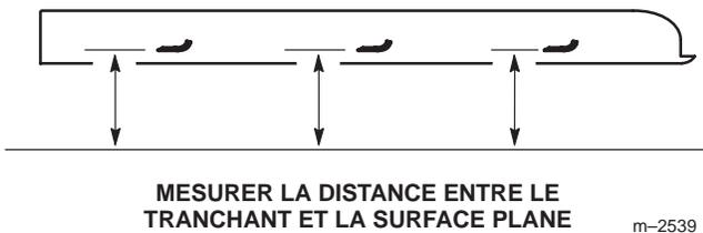
MESURER LA DISTANCE ENTRE LE TRANCHANT ET LA SURFACE PLANE
