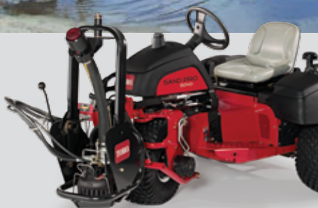
Bunker Pump, mounted on front QAS of the Sand Pro® 5040
