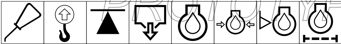
Oil lubrication point Lift point Jack or support point Draining/emptying Engine lubricating oil Engine lubricating oil pressure Engine lubricating oil level Engine lubricating oil filter
