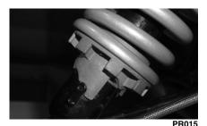
The rear shock absorber has a spring force adjustment nut with an infinite adjustment from softest to most firm. If the spring action is too soft or too stiff, adjust the nut using an appropriate spanner as illustrated.
