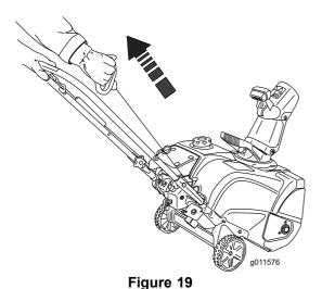
Important: Run the electric starter no more than 10 times at intervals of 5 seconds on, then 5 seconds off. Running the electric starter extensively can overheat and damage it. If the engine does not start after this series of attempts, wait at least 40 minutes to allow the starter to cool before attempting to start it again. If the engine does not start after the second series of attempts, take the machine to an Authorized Service Dealer for service (electric start only).
