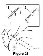
The wear-indicator hole is intact; you do not need to replace the rotor blades. The wear-indicator hole is exposed; replace the rotor blades and scraper.
