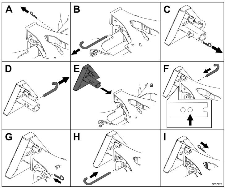
**Note:** You may need to use the front hole in the tube for some attachments; refer to the *Operator's Manual* or *Installation Instructions* for the attachment.
