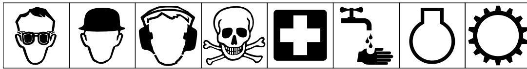
Eye protection must be worn Head protection must be worn Hearing protection must be worn Caution, toxic risk First aid Flush with water Engine Transmission
