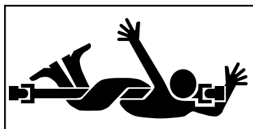
WHOLE BODY ENTANGLEMENT, IMPLEMENT INPUT DRIVE LINE
