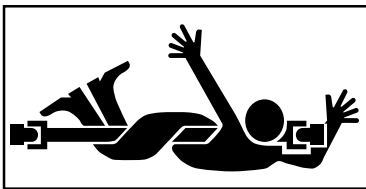
WHOLE BODY ENTANGLEMENT, IMPLEMENT INPUT DRIVE LINE
