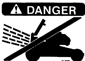
Never open discharge door on mower when engine is running, unless grass bag is installed
