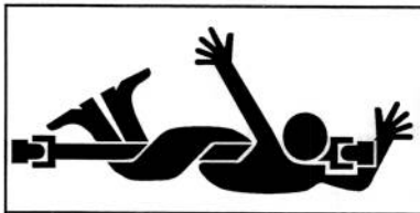
WHOLE BODY ENTANGLEMENT, IMPLEMENT INPUT DRIVE LINE
