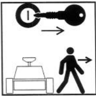
SHUT OFF ENGINE & REMOVE KEY BEFORE LEAVING OPERATOR POSITION, GREENS AERATOR
