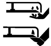
To avoid blade failure when mulching, use blade stiffener when mower is equipped with mulching plug.
