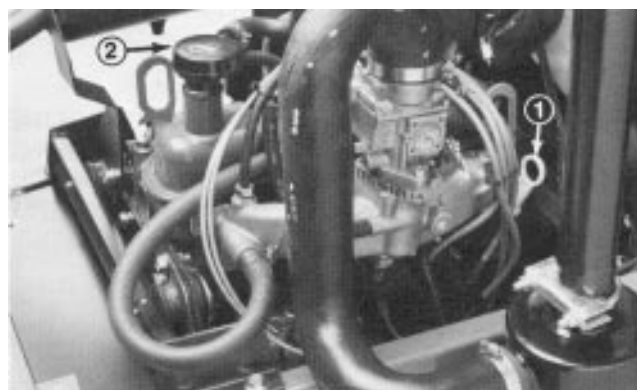
Figure 15 1. Oil dipstick 2. Filler cap
