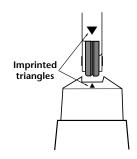
6. Align the side of the stake with the imprinted triangle to the top of the fixture head with the imprinted triangle.
