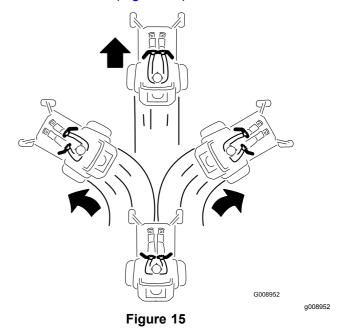
To go straight, apply equal pressure to both motion-control levers (Figure 15).
