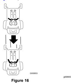
To go straight, apply equal pressure to both motion-control levers (Figure 16).
