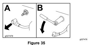
**Note:** Due to the deep recess around the spark plug, blowing out the cavity with compressed air is usually the most effective method for cleaning. The spark plug is most accessible when the blower housing is removed for cleaning.
