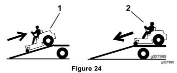
1. Back the machine up the<br/>ramp.2. Drive the machine forward<br/>down the ramp.
