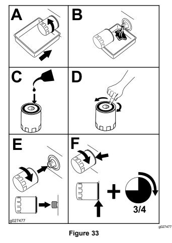
**Note:** Ensure that the oil-filter gasket touches the engine and then turn the filter an extra 3/4 turn.
