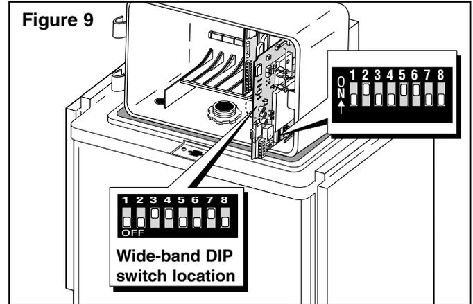
**Example for wide-band radio:** To set satellite address number 50 (050), start with all eight DIP switches in the Off (open) position, then close switch numbers 3, 4 and 7; i.e.,  $32$  (Sw 3) +  $16$  (Sw 4) +  $2$  (Sw 7) =  $50$ . See switch address code matrix in **Table 2**.
