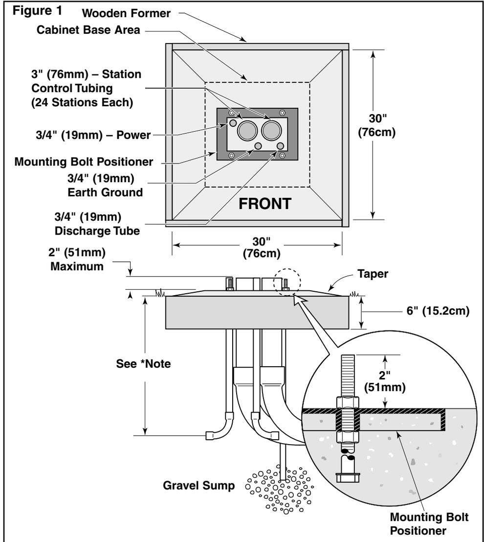
7. Finish the concrete with a level flat area of 16" x 16" (41cm x 41cm) for the pedestal base. To prevent pooling at the base of the pedestal, add a slight taper away from the cabinet base contact area. Allow concrete to sufficiently harden before continuing.
