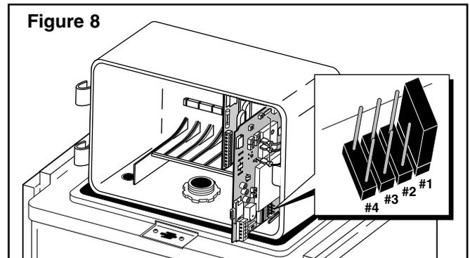
**⚠ Important:** The base station transmitter, hand-held radio and frequency decoder module must be set to the same frequency to enable communication.
