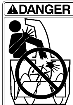
ON CHUTE (Toro Part No. 94-8079) • CONTACT WITH MOVING PARTS INSIDE CHUTE WILL CAUSE SERIOUS INJURY. • SHUT OFF ENGINE BEFORE UN-CLOGGING DISCHARGE CHUTE. • NEVER PUT HAND IN CHUTE.
