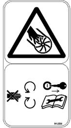
**LOW SPEED AUGER HAS MOVING PINCH POINT, CLOSE TO OPENING**
