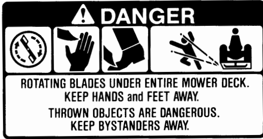
ON BOTH SIDES OF CUTTING UNIT (Part No. 66-1340) (Part No. 93-7824 for CE)
