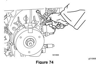
4. Check the condition of the wire-harness leads, connectors, and terminals. Clean or repair them as necessary.
