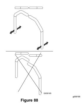
5. If the ends of the levers hit against each other, refer to Adjusting the Motion-Control Neutral-Lock Pivot (page 64).
