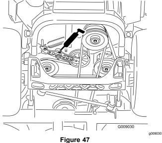
Remove the dust cap and adjust the caster pivots.
