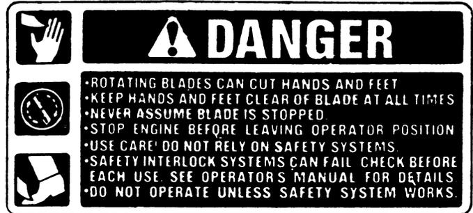
LOCATED ON FRAME PLATE UNDER STEERING WHEEL
