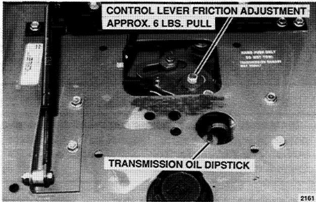
**Hydrostatic Transmission Dipstick**
