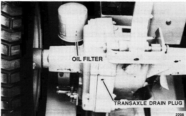
**Transaxle Drain Plug and Oil Filter**
