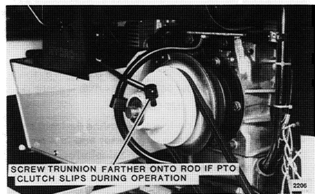
Belt Routing - Both belt strands INSIDE Rod Housing
