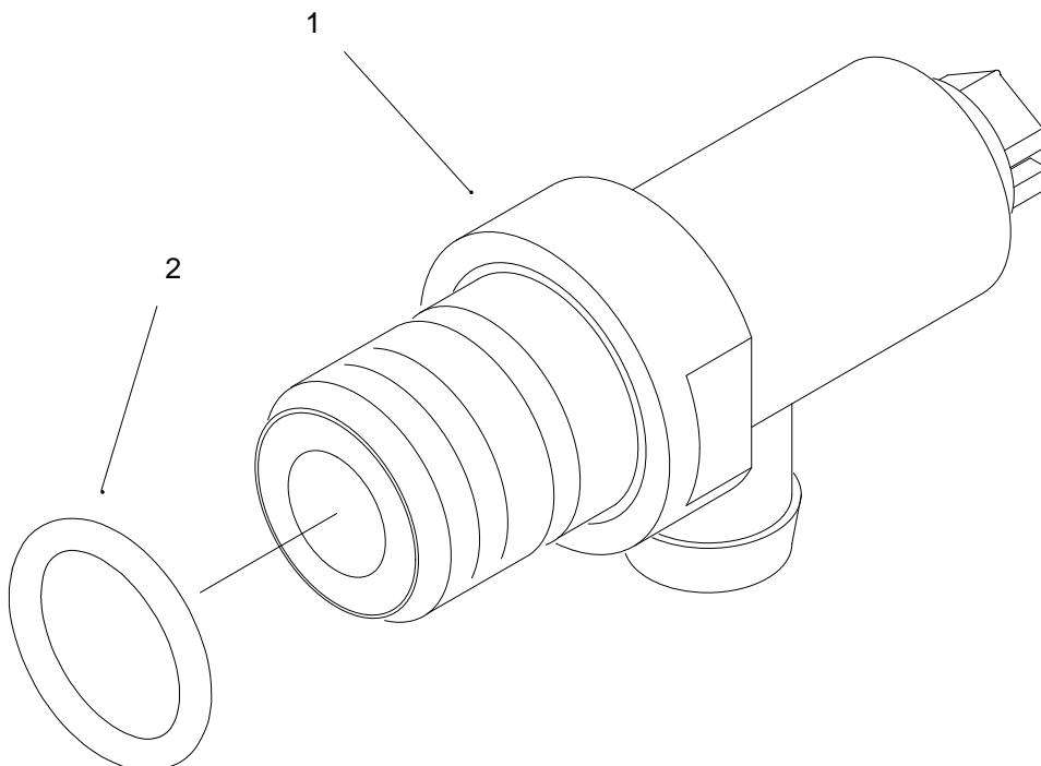
**OIL DRAIN VALVE ASSEMBLY**
