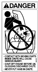
On Discharge Chute (Toro Part No. 94-8079)
