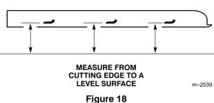
2. Rotate the opposite ends of the blades forward. Measure from a level surface to the cutting edge of the blades at the same position as in step 1 above. The difference between the dimensions obtained in steps 1 and 2 must not exceed 1/8" (3 mm). If this dimension exceeds 1/8" (3 mm), the blade is bent and must be replaced. Refer to Removing the Blades, and Installing the Blades on page 35.
