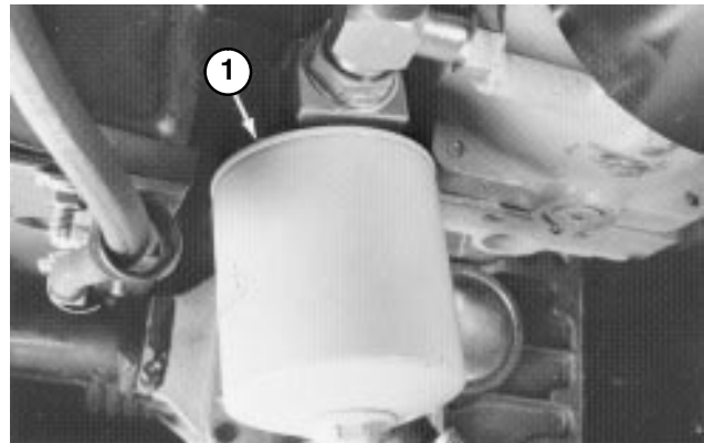
Figure 65 1. Hydraulic oil filter
