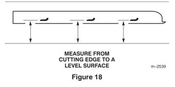
3. Rotate the opposite ends of the blades forward. Measure from a level surface to the cutting edge of the blades at the same position as in step 1 above. The difference between the dimensions obtained in steps 1 and 2 must not exceed 1/8" (3 mm). If this dimension exceeds 1/8" (3 mm), the blade is bent and must be replaced. Refer to Removing the Blades, and Installing the Blades on page 38.
