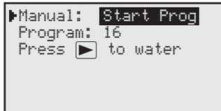
**Note:** An irrigation program must be configured to activate Manual Program. A program on hold can still be manually activated.
