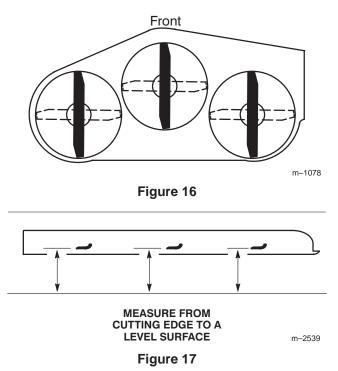
Rotate the opposite ends of the blades forward. Measure from a level surface to the cutting edge of the blades at the same position as in step 1 above. The difference between the dimensions obtained in steps 1 and 2 must not exceed 1/8" (3 mm). If this dimension exceeds 1/8" (3 mm), the blade is bent and must be replaced. Refer to Removing the Blades, and Installing the Blades on page 39.
