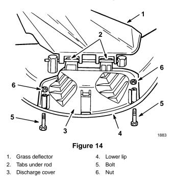
**3.** To convert back to a side discharge mower, remove the discharge cover and lower the grass deflector over the discharge opening.
