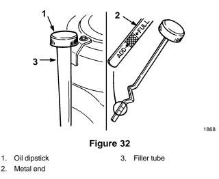
7. Slowly pour approximately 80% of the specified amount of oil into the filler tube (Fig. 32). Now check the oil level; refer to Checking Oil Level, page 33, steps 4–5.
