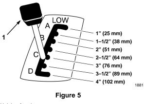
Height-of-cut lever (deck lift)
