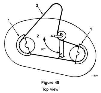
1. Pulley cover 3. Mower belt Idler pulley belt guide position
