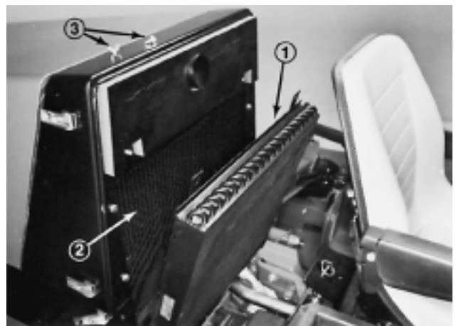
Figure 41 1. Oil Cooler 2. Radiator 3. Wing Nuts
