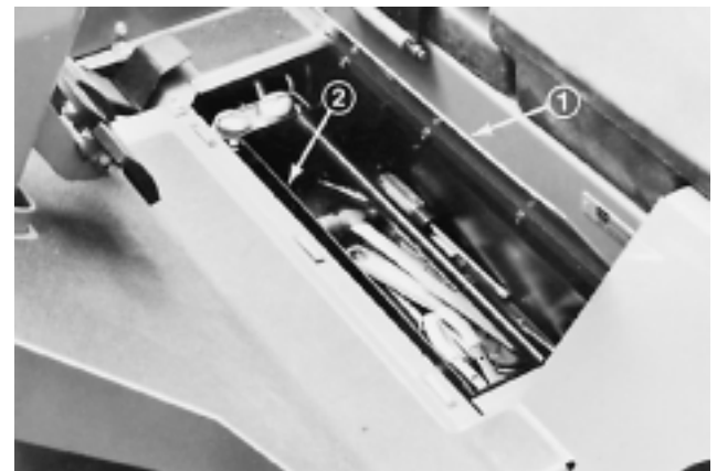
Figure 20 1. Hinged Floor Plate 2. Removable Tool Tray
