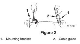
**4.** Install the right end of the lower handle onto the pin on the right handle mounting bracket (Fig. 2).
