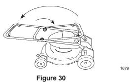
**3.** Loosen the knobs that secure the top handle section to the bottom section and fold the top handle section back toward the rear of the mower into the storage position (Fig 30).
