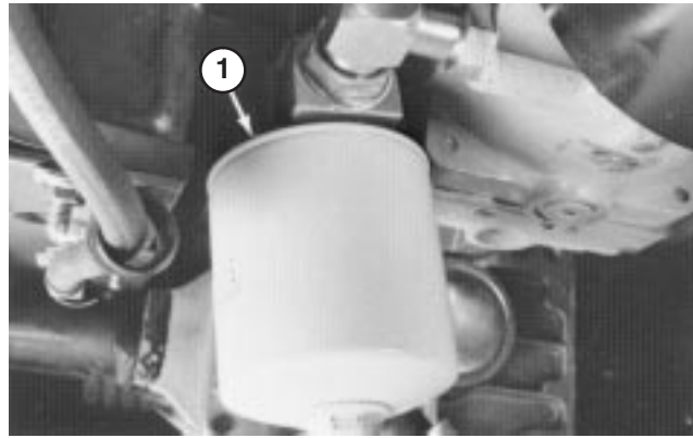
Figure 60 1. Hydraulic oil filter
