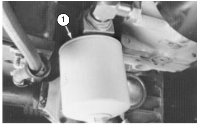
Figure 60 1. Hydraulic oil filter
