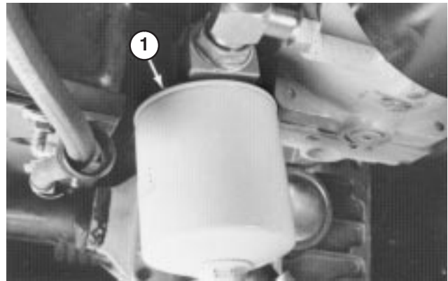
Figure 64 1. Hydraulic oil filter
