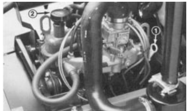
Figure 15 1. Oil dipstick 2. Filler cap
