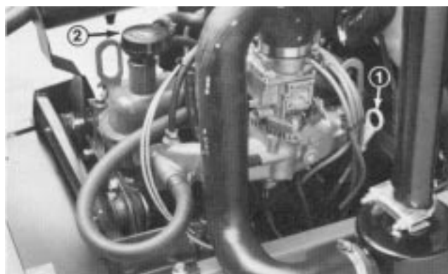
Figure 15 1. Oil dipstick 2. Filler cap
