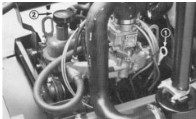
Figure 15 1. Oil dipstick 2. Filler cap
