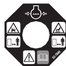
ON RADIATOR CAP (Part No. 93-7840)
