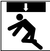
CRUSHING OF WHOLE BODY, APPLIED FROM ABOVE
