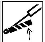
SECURE LIFTING CYLINDER WITH LOCKING DEVICE BEFORE GETTING IN HAZARDOUS AREA
