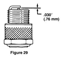
IMPORTANT: A cracked, fouled, dirty or otherwise malfunctioning spark plug must be replaced. Do not sand blast, scrape, or clean electrodes by using a wire brush because grit may eventually release from the plug and fall into the cylinder. The result is usually a damaged engine.
