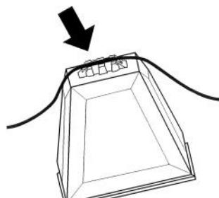
**Attach the electrical cable to the fixture.**
