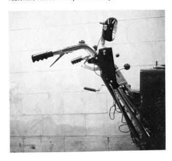
Using wire retainers, secure wire to handle.
