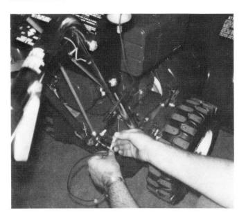
Pivot bracket and light assembly upward and resecure to escutcheon plate and handle using fasteners removed in previous step.
