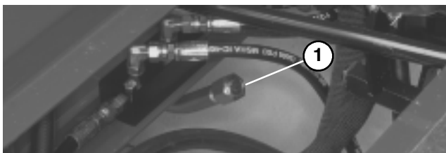
Figure 18 1. Transmission Dipstick Cap
