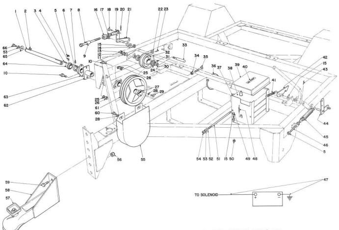
JACKSHAFT AND LIFTING MECHANISM (Model 07073) (Continued)
