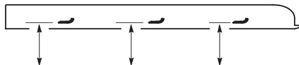
MESURER LA DISTANCE ENTRE LE TRANCHANT ET LA SURFACE PLANE
