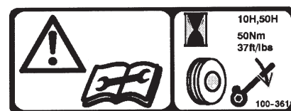
On crank pulley (Part No. 100-3611) Re-torque Taper Lock @ 10 hours and 50 hours
