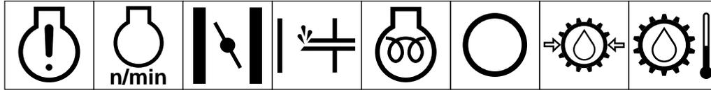
Engine failure/malfunction   Engine rotational speed/frequency   Choke   Primer (start aid)   Electrical preheat (low temperature start aid)   Transmission oil   Transmission oil pressure   Transmission oil temperature
