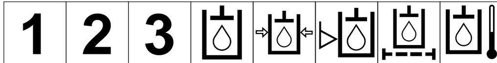
First gear   Second gear   Third gear (other #'s may be used until the maximum # of forward gears is reached.)   Hydraulic oil   Hydraulic oil pressure   Hydraulic oil level   Hydraulic oil filter   Hydraulic oil temperature
