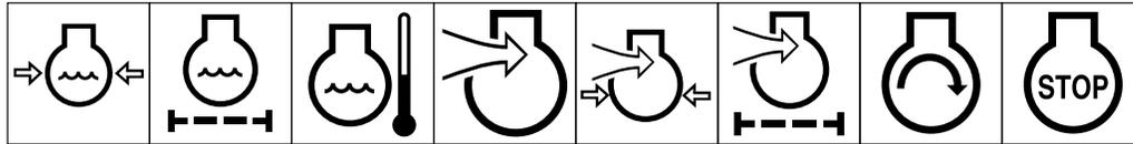
Engine coolant pressure   Engine coolant filter   Engine lubricating oil pressure   Engine intake/combustion air   Engine intake/combustion air pressure   Engine intake/air filter   Engine start   Engine stop
